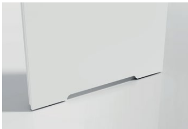
VENTILATION UNDERCUT IN PANEL DOORS 1 undercut 15 mm - for rooms with recuperation undercut 26 mm - WC for doors 80'-100' undercut 38 mm - WC for doors 60'-70'
